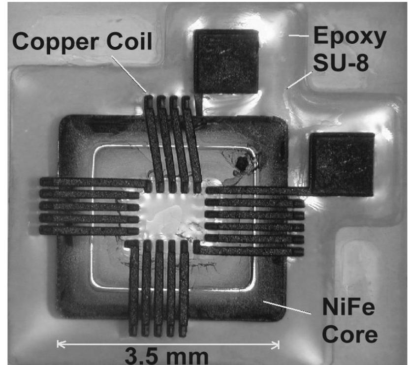
*Photomicrograph (top view) of integrated inductor with laminated NiFe core*
