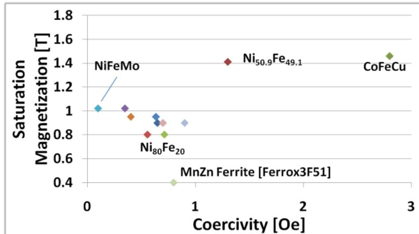
Saturation magnetization and coercivity of electroplated films
