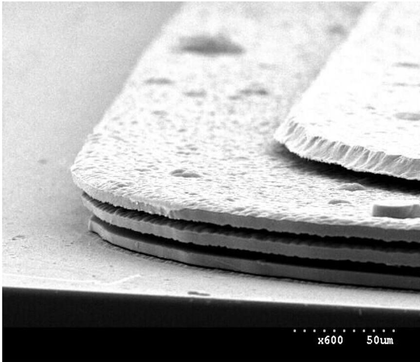
*SEM of laminated NiFe core structure after Cu removal (Detail)*
